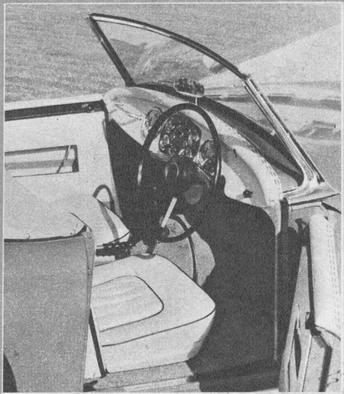
COCKPIT is well planned, beautifully upholstered, with padded leather protection round the edges, including top of dash. Rev counter is at left, gauges in centre, speedo at right. Stubby gear lever, between-seats handbrake fall readily to hand, and there's a grab-handle for the passenger.
