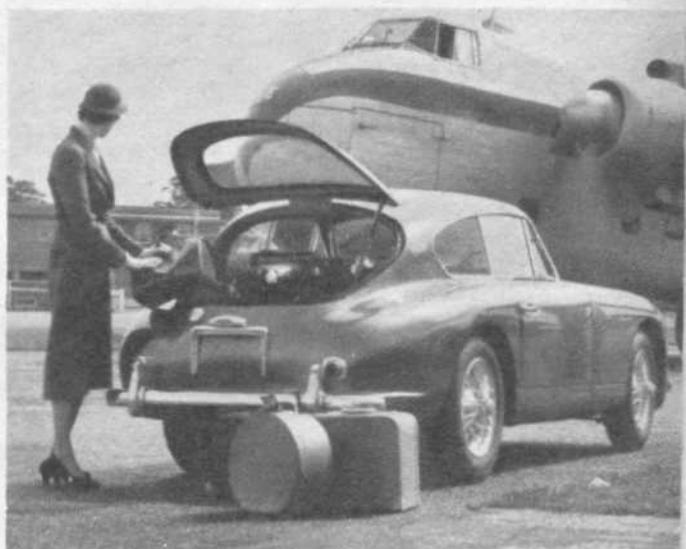
ASTON MARTIN.—The problem of good visibility and easy access to luggage on a sports body with sloping tail has been cleverly solved on the DB2-4. The photograph also shows the large side window area with thin divisions.
