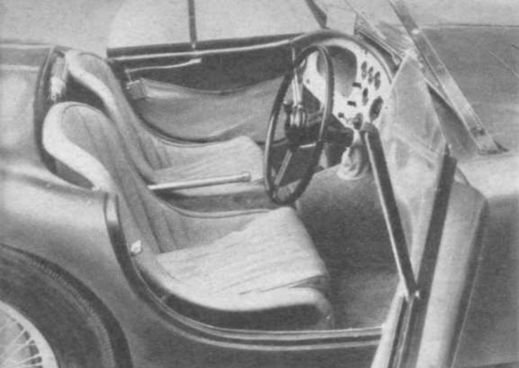
A.C. ACE.—Armchair type seats give good lateral support and a central racing type hand-brake is close to the gear lever (almost hidden by the wheel).
