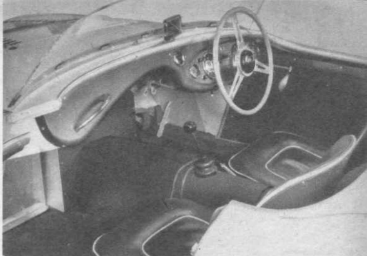
AUSTIN-HEALEY.—Notable details of the new 100S competition model include a wood-and-light-alloy steering wheel, grouped instruments in front of the driver, closely adjacent gear and brake levers, and a single-piece curved Perspex screen.
